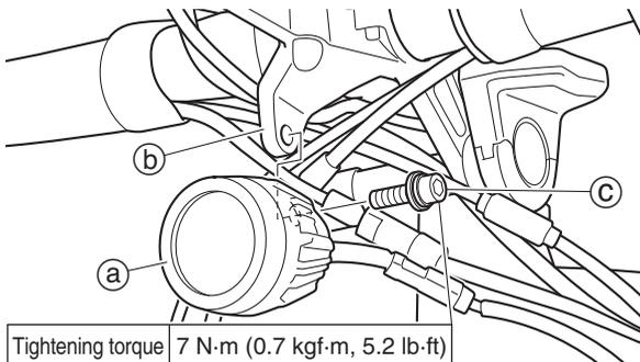
Tightening torque 7 N·m (0.7 kgf·m, 5.2 lb·ft)
