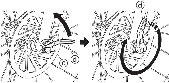
Move the lever ④ of the front axle ② to “OPEN” facing the notch ⑤.
