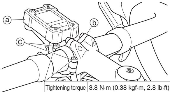
Tightening torque 3.8 N·m (0.38 kgf·m, 2.8 lb·ft)
