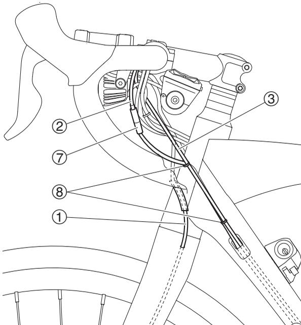
Check that the rear brake hose ②, rear shift wire ③ and speed sensor lead ⑨ are routed as shown in the illustration.
