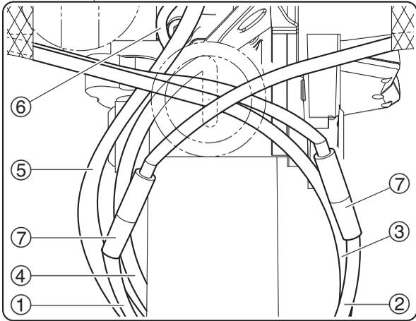
Check that the front brake hose ①, headlight lead ④, display unit lead ⑤ and plastic locking ties ⑧ are placed as shown in the illustration.
