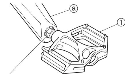
Tightening torque 40 N·m (4.0 kgf·m, 30 lb·ft)
