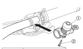
Tightening torque 0.8 N·m (0.08 kgf·m, 0.59 lb·ft)
