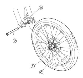
Tightening torque 11 N·m (1.1 kgf·m, 8.1 lb·ft)
