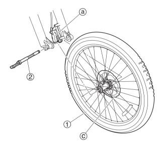
Move the lever (d) of the front axle (2) to "OPEN" facing the notch (e).
