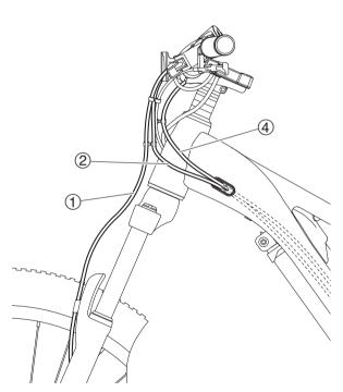
Make sure that the front brake hose 1, rear brake hose 2, and shift wire 4 are routed as shown.
