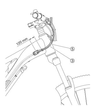
Make sure that the dropper seat wire ③ and compact multifunction meter lead ⑤ are routed as shown.
