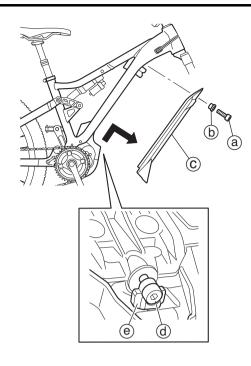
13. Installing the battery pack
