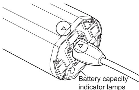
3. Unhook the claw, and then remove the battery from the battery cover.
