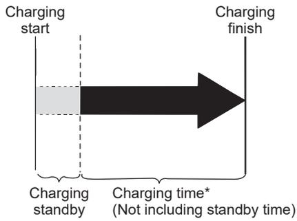
Although charging time varies depending on residual battery capacity and external temperature, if the battery has been exhausted, it generally takes approximately 4 hours (500 Wh).
