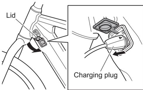
4. Confirm that charging is complete, and then disconnect the charging plug from the charging port on the frame.
